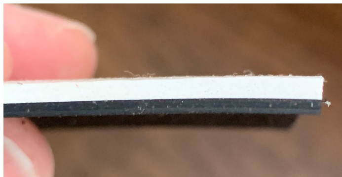
45-50 mil fluid-applied membrane on existing 45 mil roof membrane
